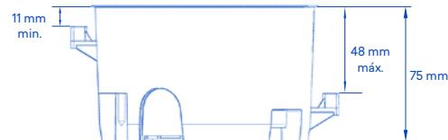
**INSTALAÇÃO EM BETÃO OU PISO TÉCNICO COM CAIXA DE ENCASTRAR | INSTALACIÓN EN HORMIGÓN OU SUELO TÉCNICO CON CAJA DE EMPOTRAR | INSTALLATION IN CONCRETE OR TECHNICAL FLOOR WITH FLUSH MOUNTING BOX | INSTALLATION DANS LE PLANCHER EN BÉTON OU TECHNIQUE AVEC BOÎTE ENCASTRÉ | INSTALLATION IN BETON ODER TECHNISCHEN ETAGE MIT UP-KASTEN**
