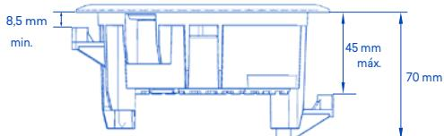
**INSTALAÇÃO EM PISO TÉCNICO | INSTALACIÓN EN SUELO TÉCNICO | INSTALLATION IN TECHNICAL FLOOR | INSTALLATION DANS LE PLANCHER TECHNIQUE | INSTALLATION TECHNISCHER BODEN**
